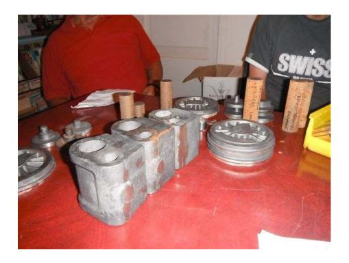
Mark unpacked a heavy box containing wheel and cylinder castings for his Speedy and cylinder castings for Ron's Springbok. Very nice castings from the UK. Ron Perkinson had problems with corrosion in the side water tanks for his PV Baker (made from zincalum or similar) and which needed replacing. He showed the parts he is preparing for fabricating new side tanks.
