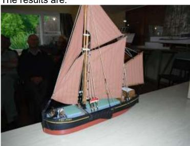
Boats: Graham Vercoe had completed building a freescale model of a Thames sailing barge from a photograph. Of balsa construction with single channel r/c and sails reasonably well with a plug-in keel. Looks very realistic.
