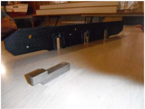
Mark Taylor showed a specially shaped drawbar for his ground level 7 1/4" passenger trolley. He also had the frames for a 5" gauge Speedy which will be his next project. Discussion on the relative merits of different axle box bearings - plain bearings, needle rollers or split bush bearings. The frames had been cut by high
